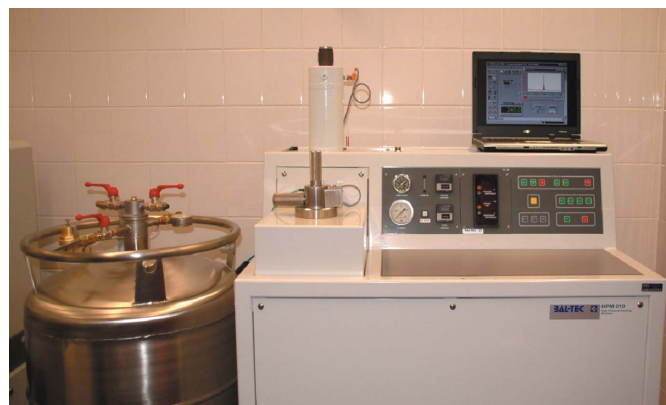
Figure 3 Baltec HPM 010 high-pressure freezing device.
